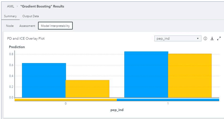
Figure 8: In blue is the ICE plot for a single transaction and in yellow is the PD plot. We can tell from our ICE plot that pep_ind had an impact on this observation's decision (around .6 probability when pep_ind = 0 vs .8 when pep_ind = 1). The PD plot shows a much bigger impact for pep_ind. This demonstrates how the global explainer (PD) can diverge somewhat from the observation-specific local explainer (ICE).
