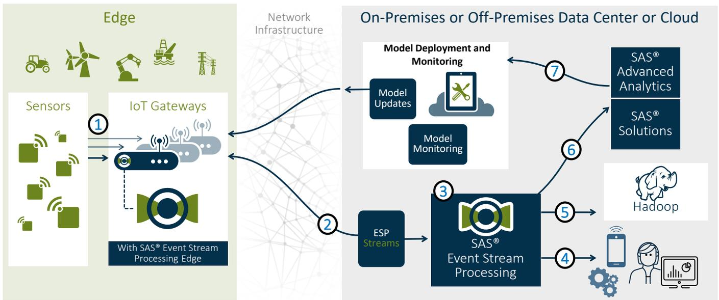
Figure 2: An Internet of Things architecture using SAS Event Stream Processing.
