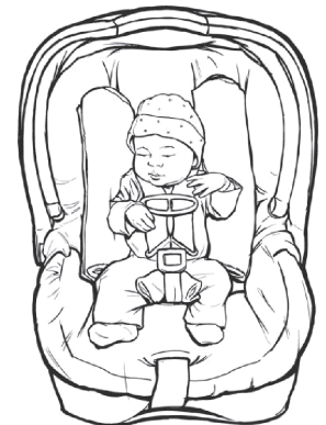
Figure 4. Car safety seat with a small cloth between crotch strap and infant, retainer clip positioned at the midpoint of the infant's chest, and blanket rolls on both sides of the infant.
