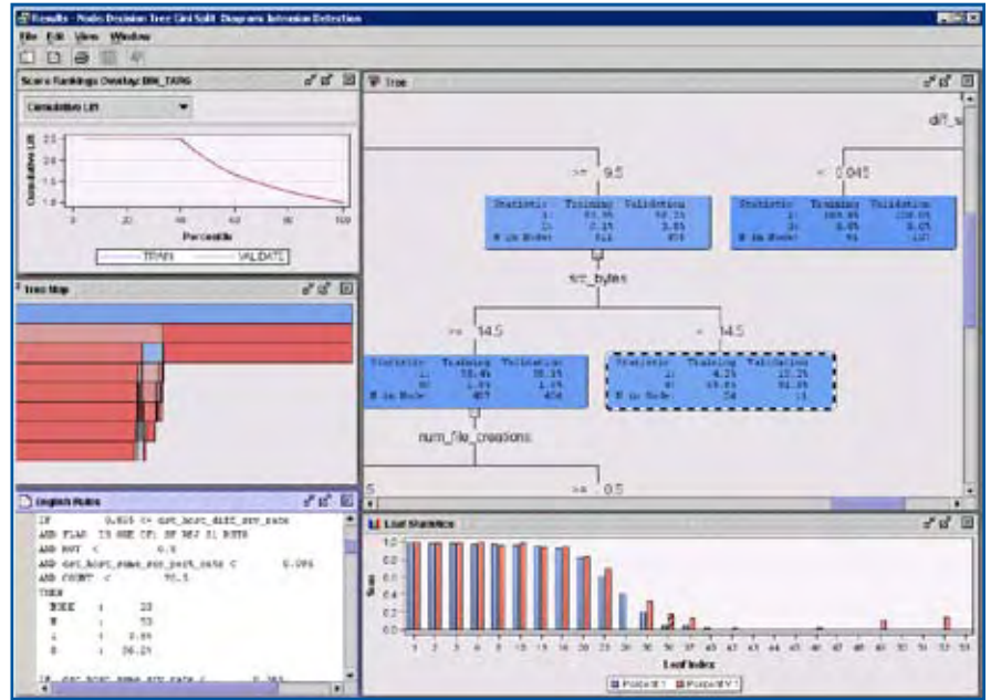
Figure 10: Develop decision trees interactively or in batch. Numerous assessment plots to help gauge overall tree stability are included.
